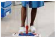
Open the mop holder by pushing the red foot-operated button
